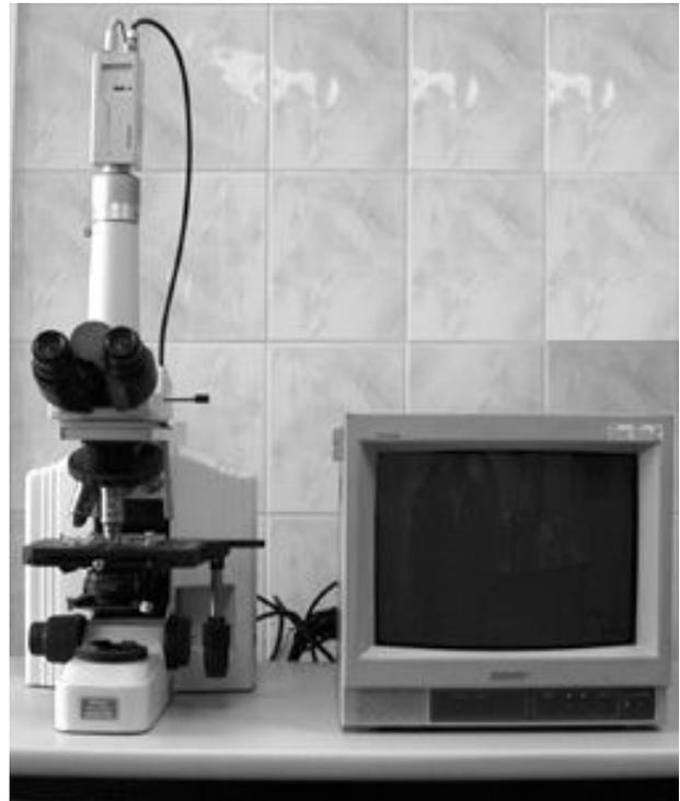
**Figure 1** | The microscope system used in this study. A light microscope (Nikon Eclipse E 600) is attached to a monitor through a CVC camera.
