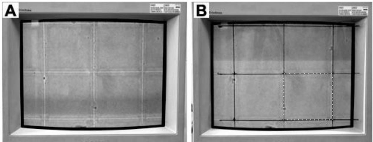
**Figure 2** | Calibration of the screen according to the Thoma Glass scale. A) The scale on the Thoma Glass was magnified with either 10, 40 or 100X objective and visualised on the screen. This image was taken with 100X objective. B) The image of the Thoma Glass scale on the monitor screen for each magnification was transferred on to an individual transparency. Unite square area shown with dashed lines equals to 0,0025 mm<sup>2</sup> in our study.
