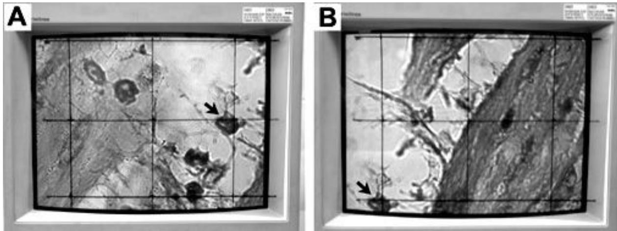
Figure 3 | Two dimensional (x-y) stepping on the stage of microscope. The reference point shown with a black arrow in panel A is moved 50  $\mu\text{m}$  in y axis and 100  $\mu\text{m}$  in x axis as shown in panel B.
